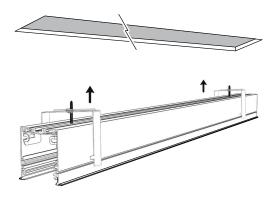
60mm Min Do not over tighten Clamp Screws
