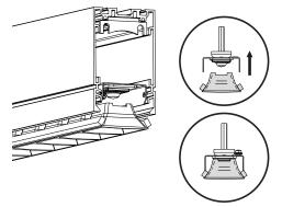
Ensure shades are fully clipped on prior to installation. Should be flat along lamp tray.
