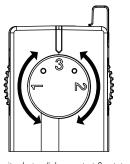
If the circuit selector dial was set at 0, rotate it to select 1, 2 or 3 depending on the circuit required for that luminaire.
