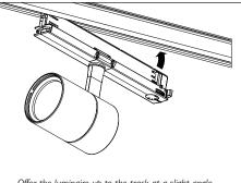
Offer the luminaire up to the track at a slight angle so that the lever and dial are slightly lower than the opposite end of the Track Adapter.
