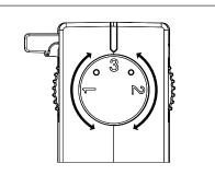
Rotate the dial to select 0 (off), 1, 2 or 3 depending on the circuit required for that luminaire, by aligning the number with the raised mark.
