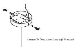
Disconnect the Earth Cable from Earth Tab.
