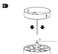
Feed Suspension Wire through Clutch while pushing down on Clutch Neck. Once released, this will support the luminaire temporarily,
