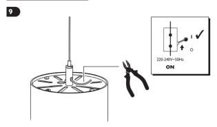
Cut away excess Suspension Wire
