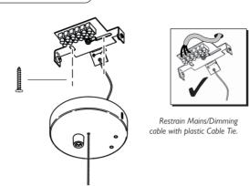
Ensure suitable fixings are used when installing.
