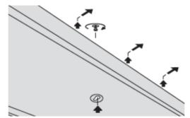
Tighten screws after installation
