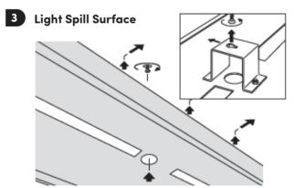
Tighten screws after installation
