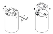
Unscrew 2x fixing screws (Do not fully remove), until luminaire can slide off and unhook.
