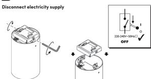
Unscrew 2x fixing screws (Do not fully remove), until luminaire can slide off and unhook.
